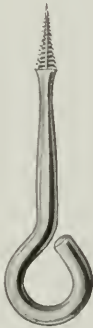
Fig. 30.—Short-Shank Screw-Porte. Without handle. The shank has a ring end for receiving a small bar as a handle.
